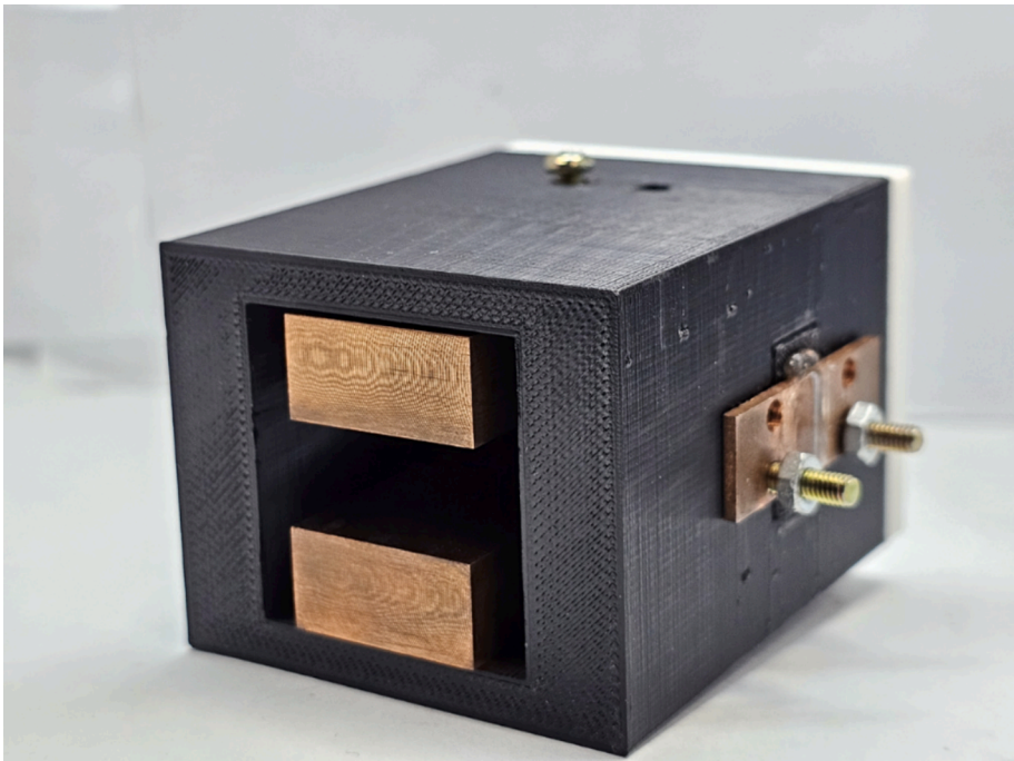
Fig. 3. Diagram of the pulsed plasma thruster.
